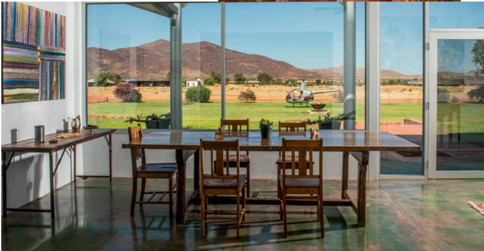
The flooring is polished concrete, made using sand from the local creek containing all sorts of rocks and pebbles in varying shapes, colours and sizes. Brad spent six weeks grinding and polishing to get the very best result.
